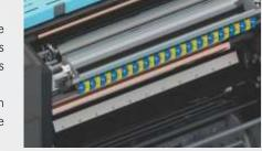
Ink roller cleaning is quickly done using pneumatically operated cleaning tray. In addition Pneumatically operated bridge roller is provided to engage the dampening rollers with ink rollers for easy washing.
